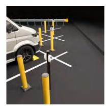
For industrial and larger public car parks, we provide 2 No. ImpactSAFE Protection Posts and a Wheel Stop for added coverage. We recommend this package as a solution when there is a medium-tohigh risk of impact damage and where light industrial vehicles (such as electric vans) are going to be using these charging points.
